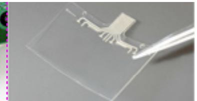
clear ITO on PET with silver connections
